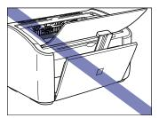
• Do not leave the top cover open for any longer than you need to. Exposure to direct sunlight or strong light can degrade the printer performance.
